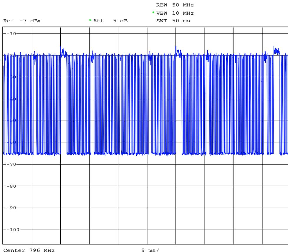
Figure B.4: Zero span plot of a 50 ms section of "LTE\_BS-idle\_V3\_synth" waveform
