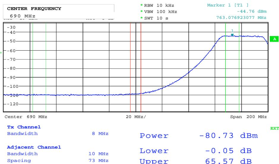
**Figure D.1: Frequency response of band pass filter used for ACLR improvement**
